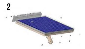
Secure bird guard to panel frame using 6 x M6 bolts.
