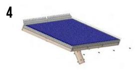
Secure Clasps using self-tapping screws along bottom edge of panel.
