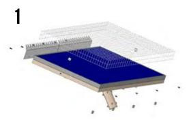
Place Solar panel Stone Guard completely over panel leaving 30-35mm clearance between mesh and solar panel glass.
