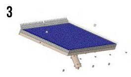
Secure clasps around edge of stone guard mesh and attch with self tapping screws.
