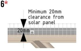
**MINIMUM CLARANCE 20mm FROM** TOP OF PANEL TO AVOID DRILLING INTO GLASS CAUSING DAMAGE.
